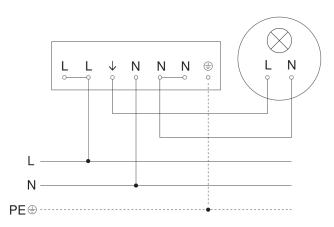
Connection using two-circuit switch for manual and automatic operation
