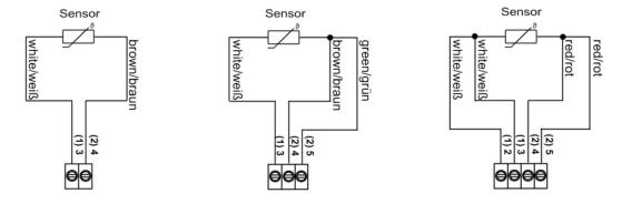
fig. (terminal assignment passive sensor)
