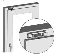
Mount the magnet flat as shown next to the arrow marking.
