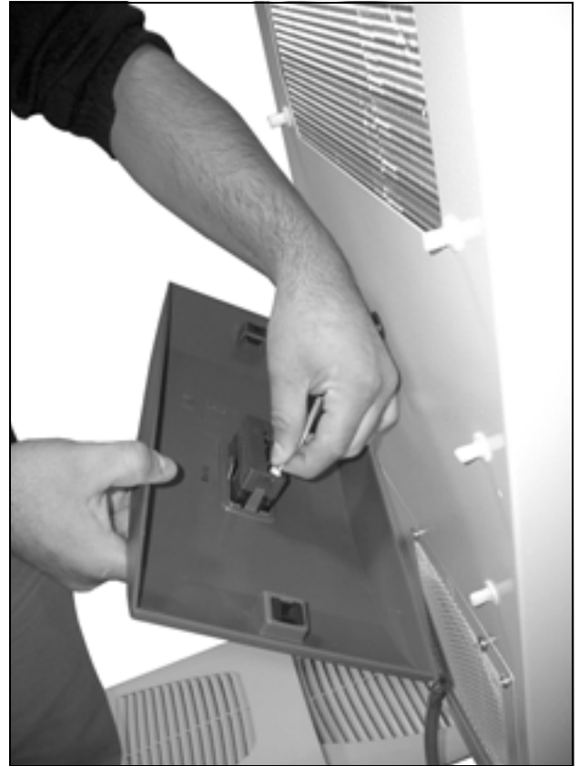
Fig. 43: Disconnect the connector from the display (1)
