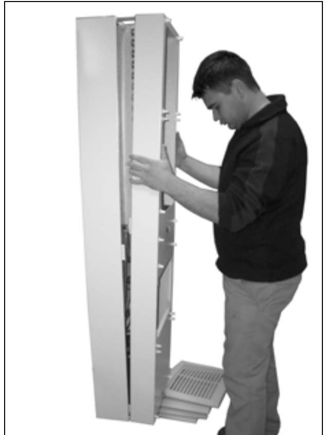
Fig. 76: Removing the cover
