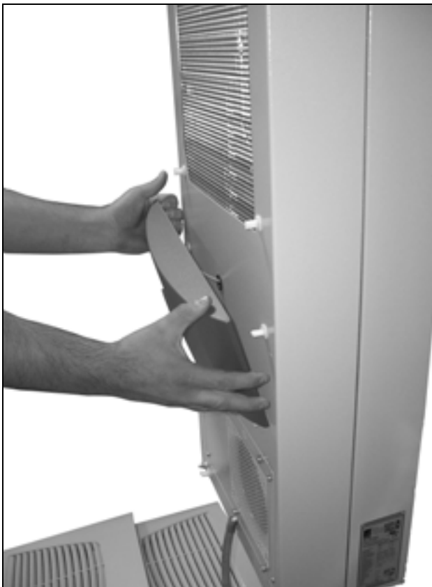
Fig. 42: Remove the infill panel
