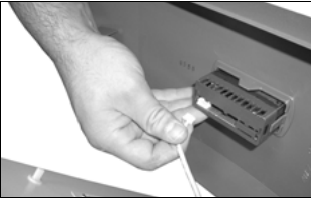
Fig. 65: Disconnect the display cable
