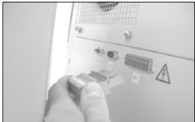
Fig. 39: Disconnect the mains plug
