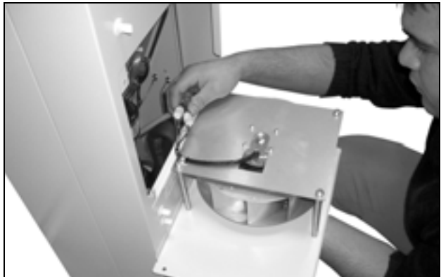
Fig. 70: Disconnect the fan connectors (1)
