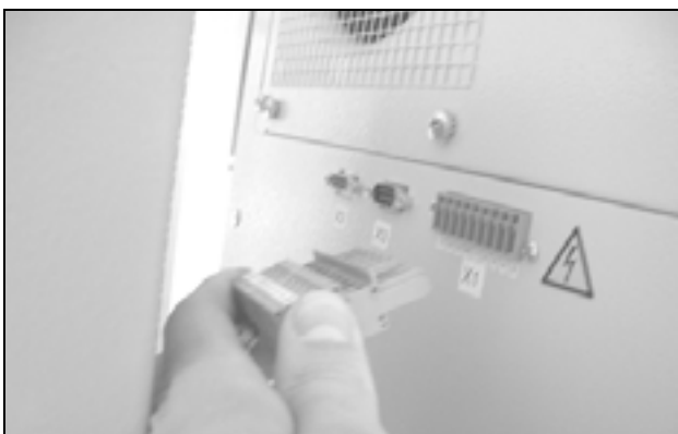
Fig. 58: Disconnect the mains plug
