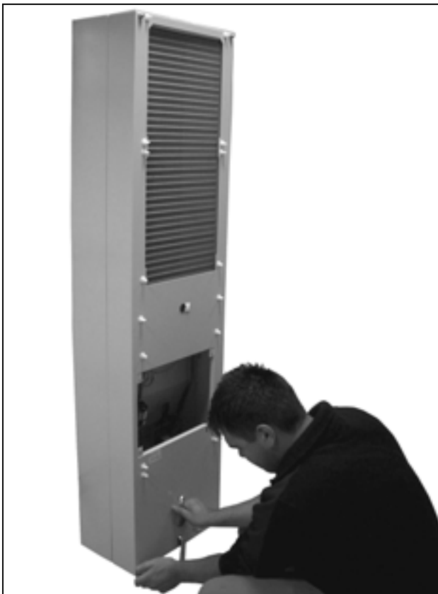
Fig. 75: Undo the four screws for the cover
