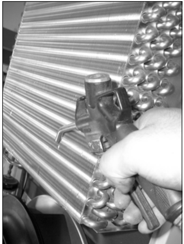
Fig. 56: Clean the heat exchanger coil and compressor chamber using compressed air (1)
