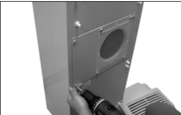
Fig. 68: Undo the four screws for the external circuit fan
