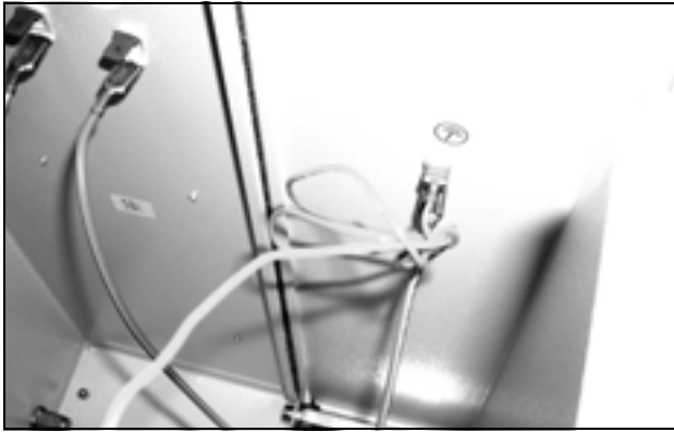
Fig. 73: Disconnect the fan earthing cable (1)
