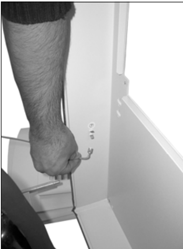
Fig. 78: Disconnect the earthing cable (2)
