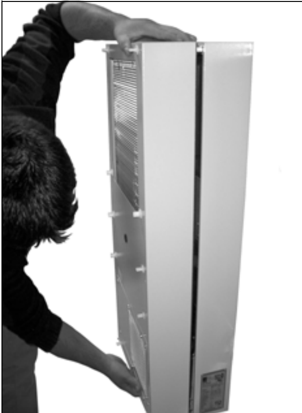
Fig. 52: Remove the cover (1)
