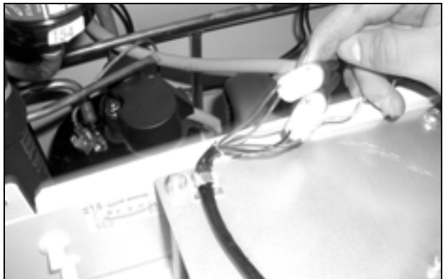
Fig. 71: Disconnect the fan connectors (2)
